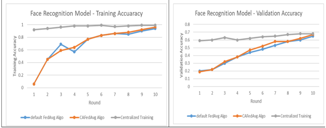
Figure 6.3: Facial recognition ML model training and validation accuracy using default FedAvg algorithm, CAFedAvg algorithm and Centralized training (#rounds=10, #epochs=10)
