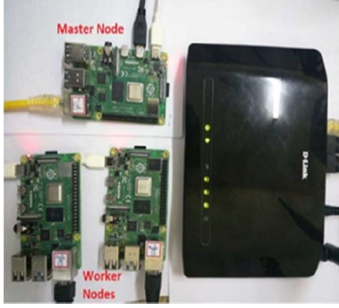
Figure 3.25: Experimental Setup of Fog Cluster with One Master Node and Two Worker Nodes
