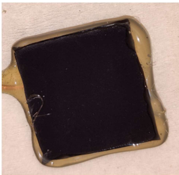
Figure 3B.5: Digital image of one of the working electrodes, used during electrochemical measurements.
