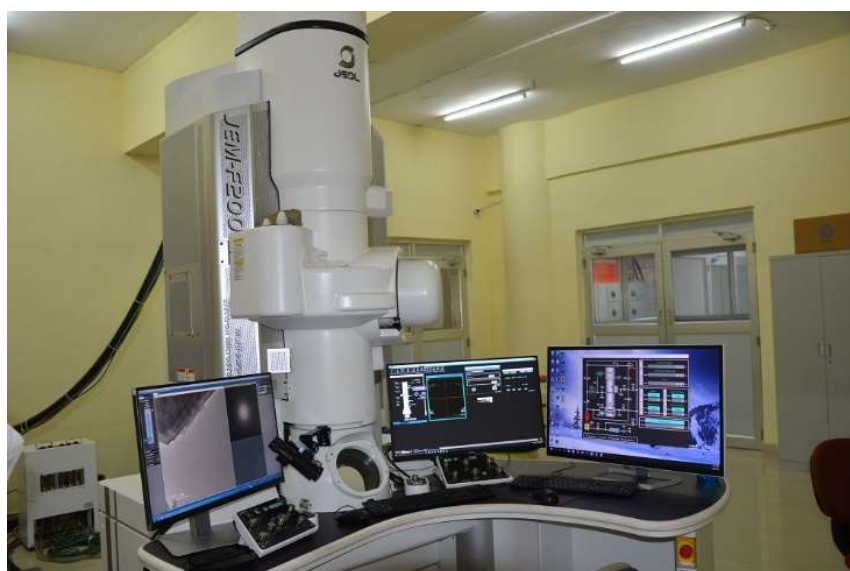
Figure 2.9: Digital image of JEM-F200, JEOL TEM.
