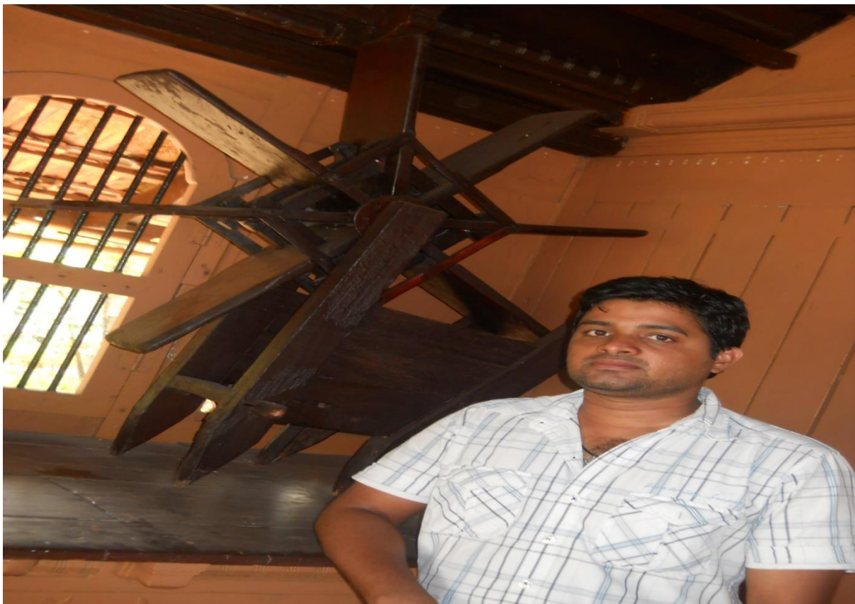
A Chakram , which was used to de-water the fields in earlier years.
