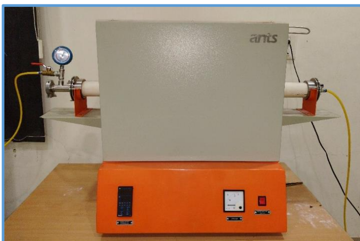
Fig. 2.12 Thermal annealing chamber (ANTS, Copper Electric 1200 Degree C Horizontal tube furnace).
