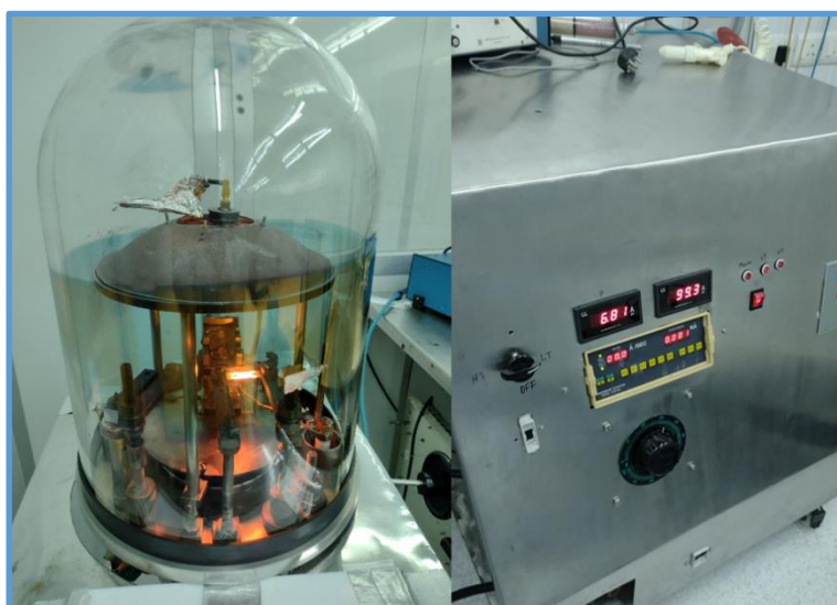
Fig. 2.11 Image of the thermal evaporation chamber and its controller used for Au deposition.
