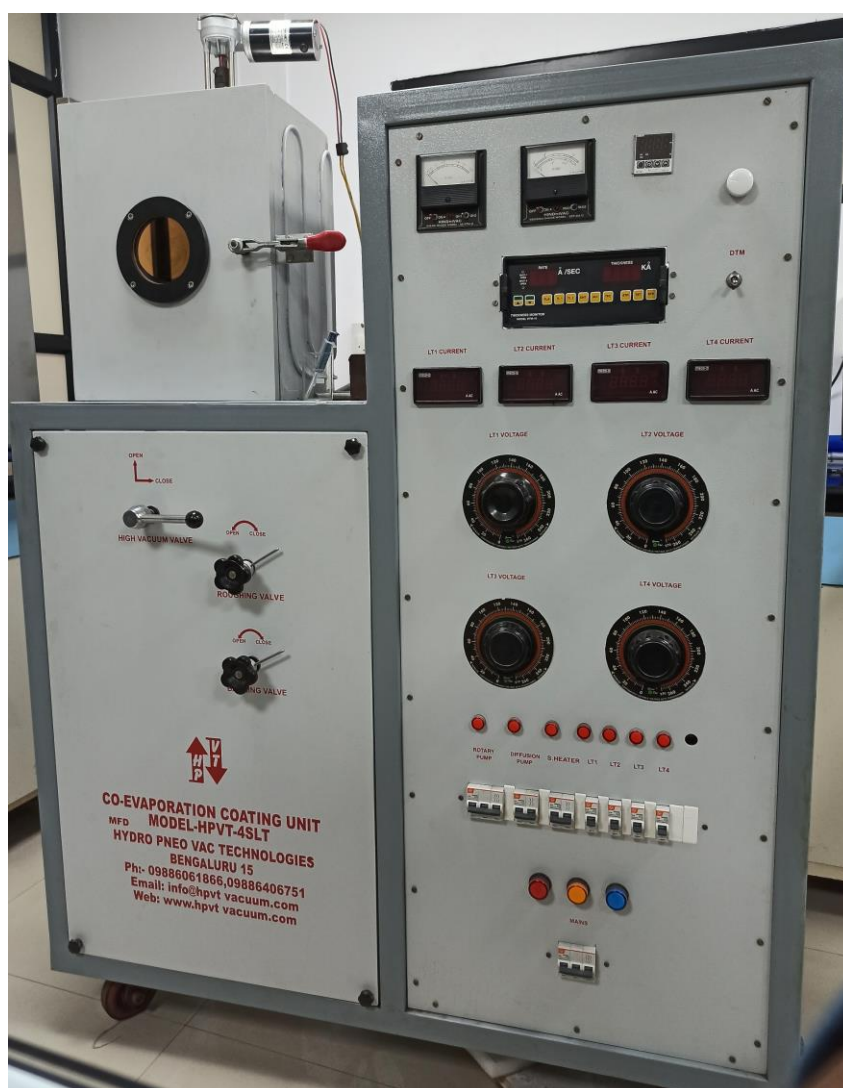
Fig. 2. 5 Photo images of thermal evaporator for gold deposition at SoC, UoH.
