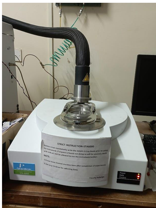
Fig. 2. 8 Thermogravimetric analyzer used for thermal properties at SoC, UoH.
