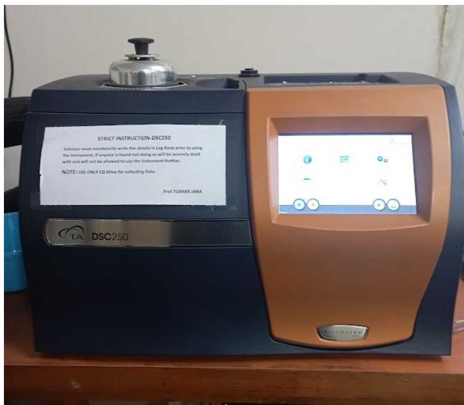
Fig. 2. 9 Differential scanning calorimetry (DSC) used for change in material behaviour with temperature at SoC, UoH.
