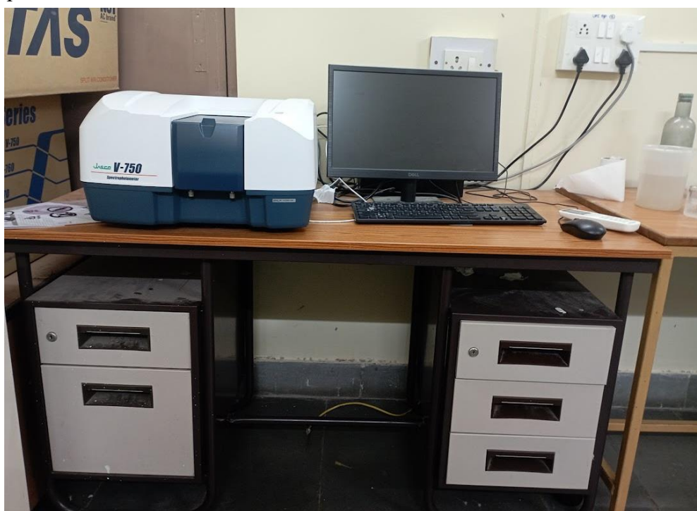
Fig. 2. 6 UV used for bandgap investigations at SoC, UoH.
