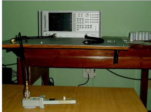
Fig 6. 5: WR-90 cavity connected to the VNA
