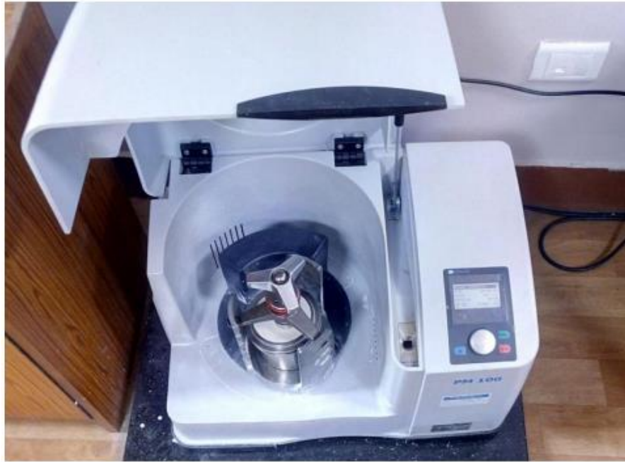
Fig 2. 1: Ball Mill with Zirconia Jar loaded
