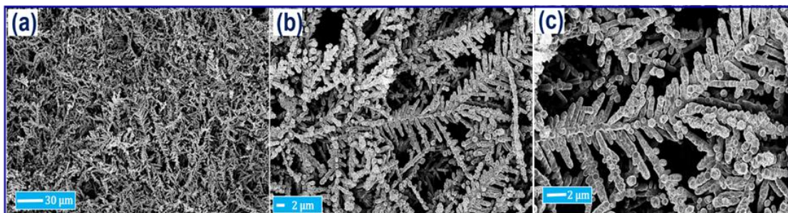
Figure 4.5: SEM images of the AuNPs (on AgNDs) decorated at 3 hours' reaction time (AuNPs deposited at 1 mM concentration) (i.e., AuNPs@AgNDs-3) viewed at different magnifications.
