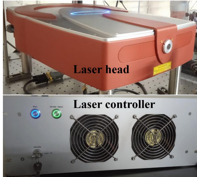
Fig. 5: The pictorial of diode pump fiber laser system comprised of laser head and controller.
