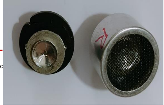
Figure 2.9: Piezoelectric ultrasonic transducer structure and representation of the transducer
