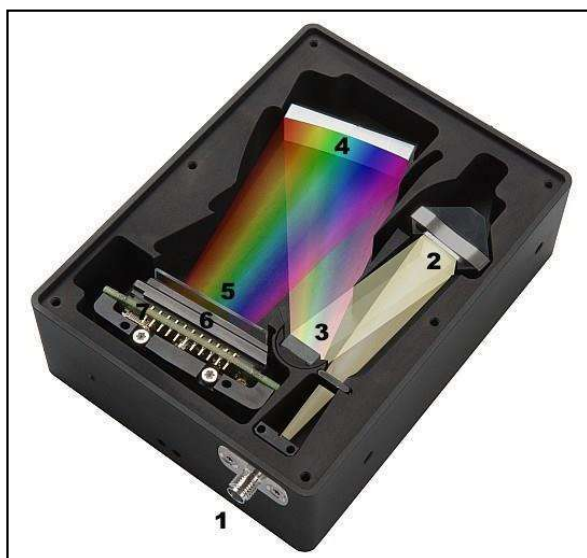
Figure 2.10 Major components of the CCD-based non-gated spectrometers from the entrance to the CCD detector and the grating and mirrors [Adopted from https://www.avantes.com/support/theoretical-background/introduction-to-spectrometers/ ].
