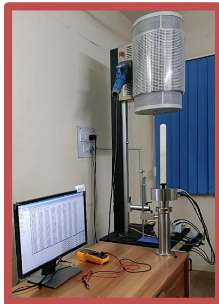
Figure 2. 10. Photograph of Dielectric property measurement system.
