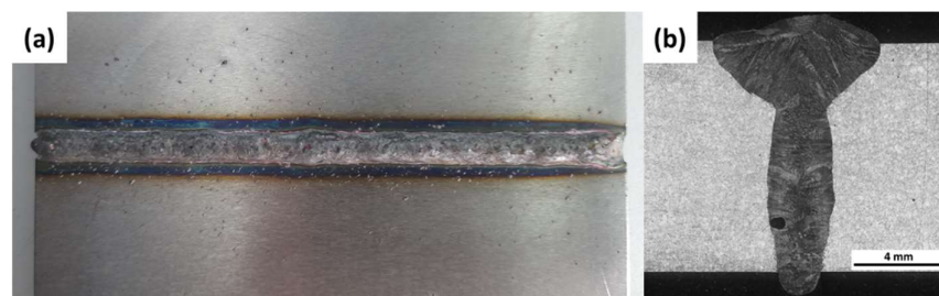
Figure 8.5. Weld obtained by novel method (a) Seam welded plate and (b) Macrograph
