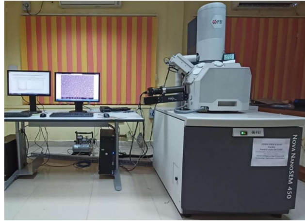
Figure 3.18. Field emission scanning electron microscope (FESEM) attached to EDS/EBSD
