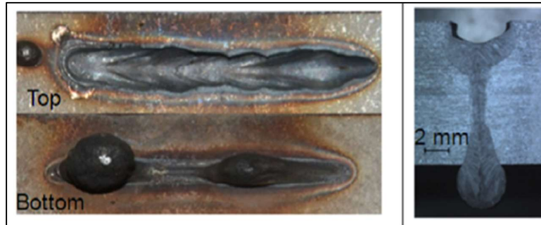
Figure 2.10. Deep-penetration laser weld top and bottom bead along with weld cross-sectional showing huge underfill and root hump defects [25]
