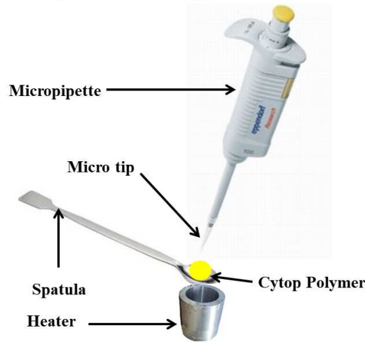
FIGURE 2.10: Droplet making through micropipette injection
