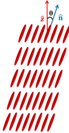
FIGURE 1.5: Schematic diagram showing Smectic-C phase. Red rods indicate calamitic molecules. \theta is the angle subtended by the director with the layer normal.
