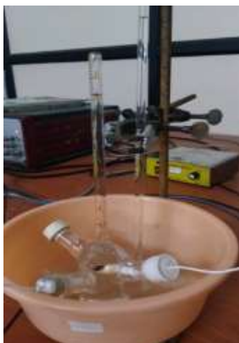
Figure 11: Set-up for quantitative hydrogen evolution.
