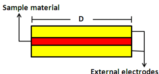
Fig. 2.4. Sample capacitor prepared with two round disposable plate electrodes.
