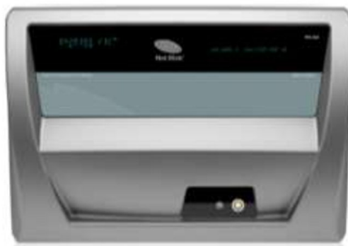
Fig 5.6 Hot Disk TPS 2200 thermal constant analyser[121]
