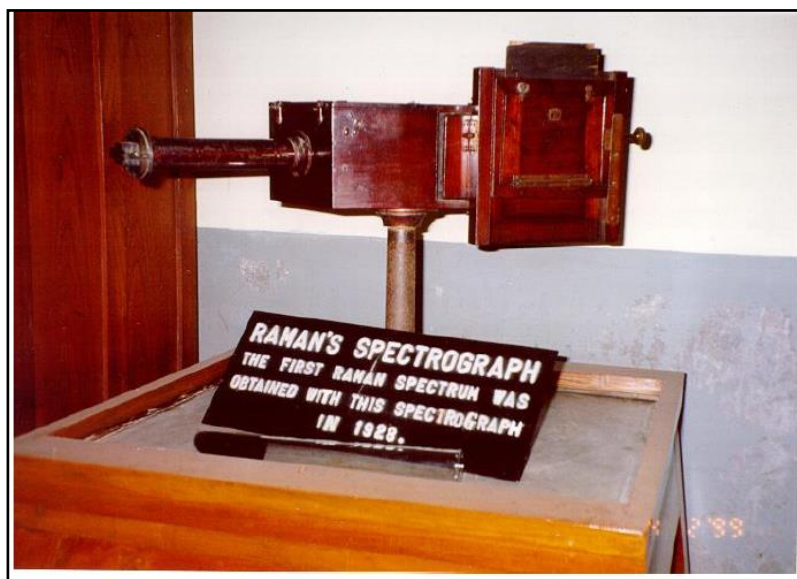
Figure 1.1 The first Raman spectrometer, built by Sir. C.V. Raman 19
