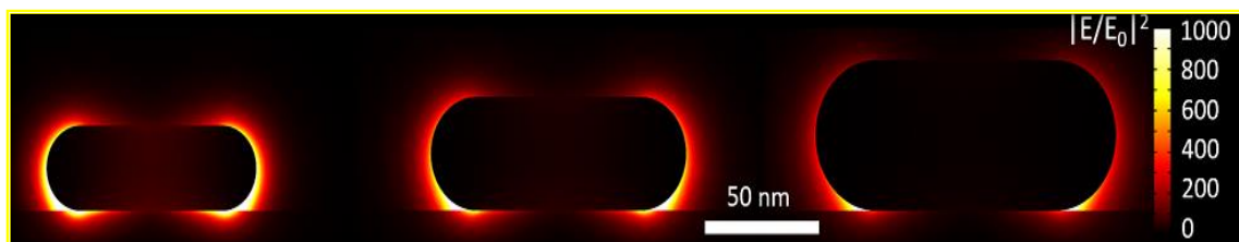
Figure 1.10 Theoretical simulated local electric fields of three different sizes Au nanorods [adopted from Lin et al.] 54
