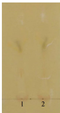
Fig. 3.3: Thin Layer Chromatography (TLC) analysis of Ent incubated with (lane 1) and without OPH (lane 2). The Ent incubated with either buffer or with OPH was extracted and spotted on TLC plate. The TLC was performed using benzene: acetic acid: water in a ratio of 62.5ml: 36ml: 1.5ml (v/v) as solvent system.
