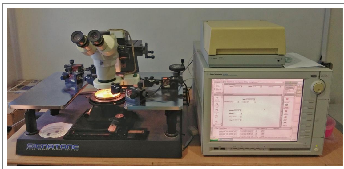
Fig. 2.22: Agilent technologies (B1500A) semiconductor device analyzer with attached Signatone probe station - P1160 at CFN, UoH [29].
