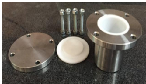
Figure 1.5. Showing a picture of an autoclave used to carry a hydrothermal reaction.
