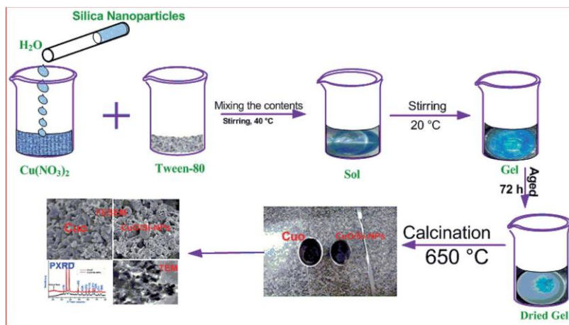
Figure 1.6. CuO nanoparticle synthesis by sol-gel technique [71].
