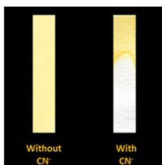
Figure 2.43. Test strip detection of CN - in water.
