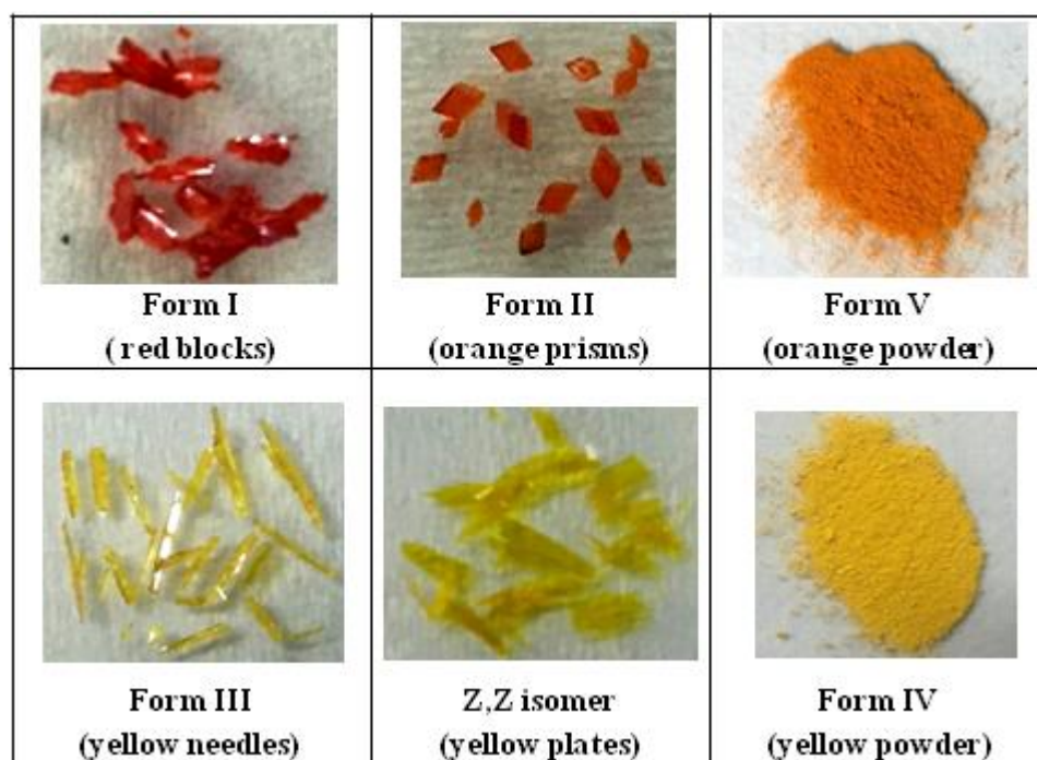
Figure 4.2 Photographs of different colored EPR polymorphs: deep red – form I, deep orange – form II, orange – form V; bright yellow – form III, yellow – form IV, and bright yellow – Z,Z isomer.
