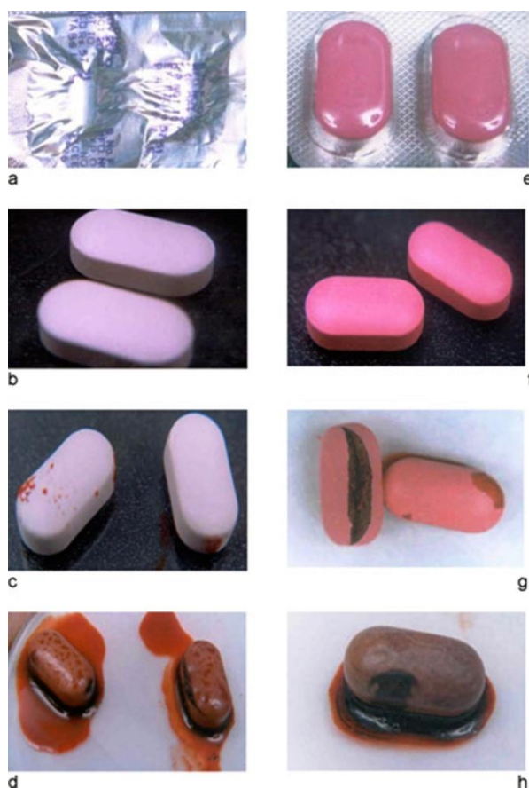
Figure 3.1: Decomposition of 4-FDC tablets (a, e) on the shelf after storage at accelerated conditions of 40 °C/ 75% RH for a period of 2 days (c, g) and 5 days (d, h).
