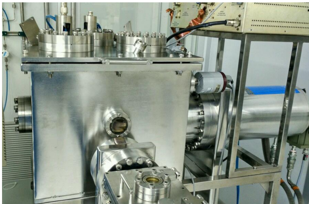
Figure.2.8. The RF magnetron sputtering system used in this study.
