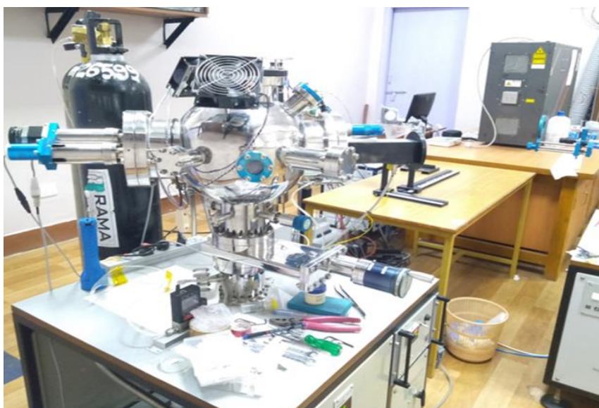
Fig. 2.6. Pulsed laser deposition (PLD) set up with high vacuum (HV) chamber.
