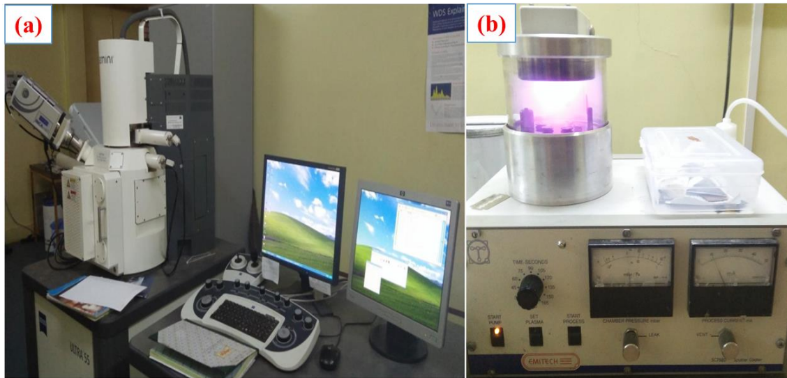
Fig.2.10 (a) Field emission scanning electron microscope (model: Carl ZEISS, Ultra55, Germany) (b) Gold coating sputtering unit for non-conducting samples.
