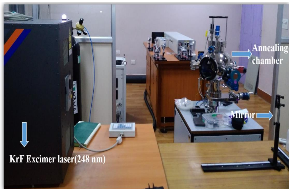
Fig. 2.8. Set-up for the laser annealing of thin films with the chamber and KrF- Excimer laser.
