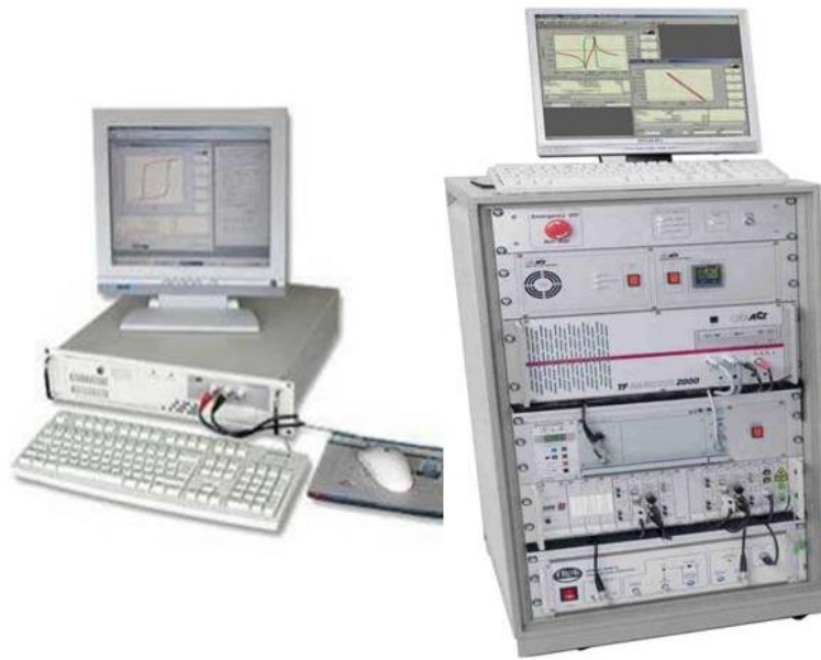
Fig. 2.16. TF 1000 Analyzer of aixACCT GMBH, Germany for leakage current measurement.
