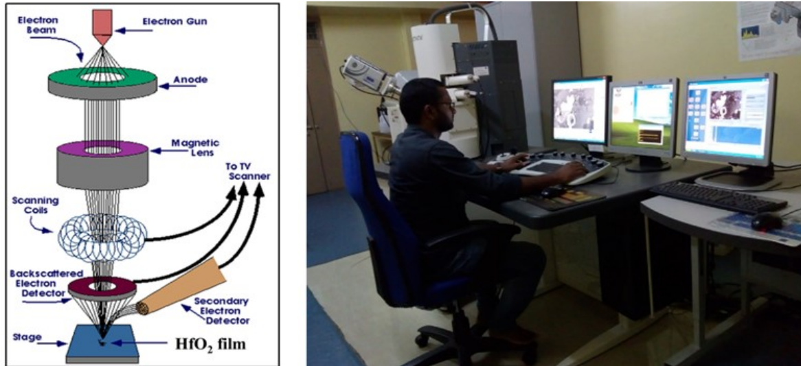
FIGURE 2.18: (a) schematic illustration of scanning electron microscopy (b) Carl ZEISS, FEG, Ultra 55 FESEM system installed at SoP, UoH.
