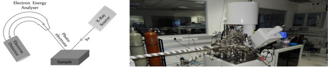
FIGURE 2.20: a) schematic of X-Ray Photoelectron Spectroscopy and b) AXIS ULTRA Multi-technique X-ray Photoelectron Spectroscopy installed at IISc, Bangalore.
