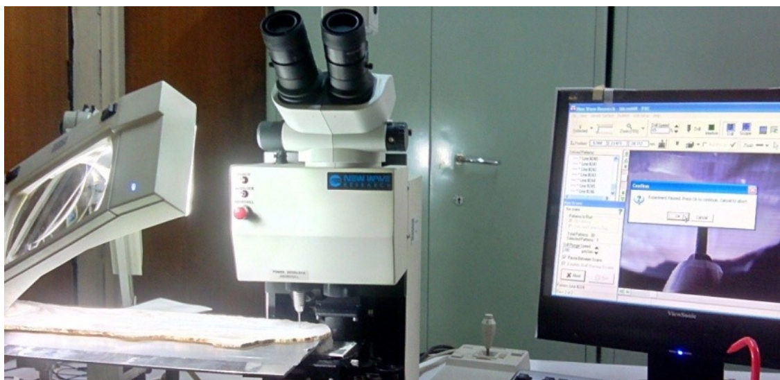
Fig. 3.3. Micromilling. Sub-samples of stalagmites KG-6 and BRA-3B were drilled using an automated New Wave Research Micro-mill at PRL, Ahmedabad.
