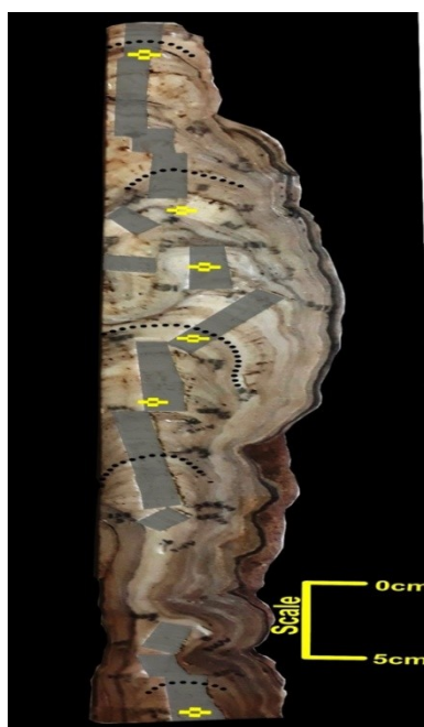
Fig. 3.5. Stalagmite Slicing for sub-sampling. Slice of BRA-3B stalagmite with showing sum-sampling along growth layers (grey). Yellow points are U-Th age points and black dotted lines are selected growth layers for Hendy's Test
