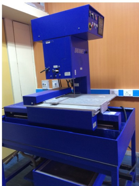
Fig. 3.1. Stalagmite Cutting. Stalagmites were cut into two equal halves and sliced for U-Th age estimations and stable isotopic analyses using Dramet cutting machine at PRL, Ahmedabad.
