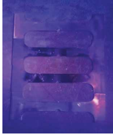
Figure 64: FLPT results captured under UV light in dark room
