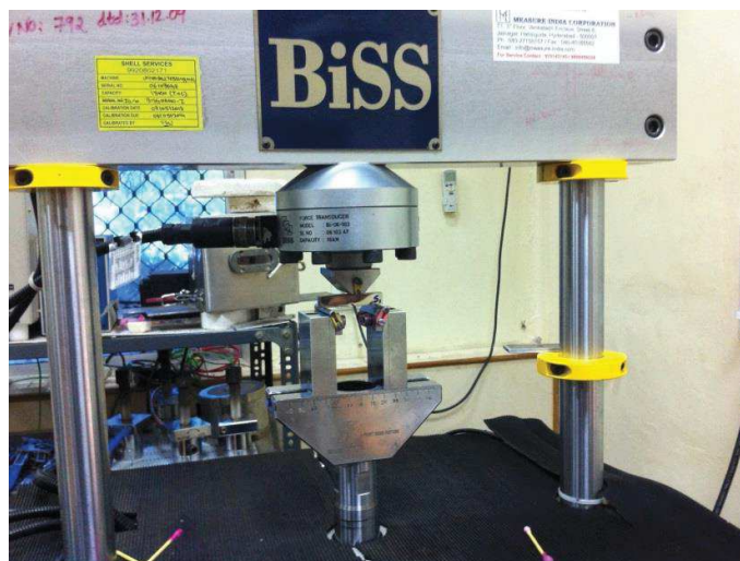
Figure 35: Experimental set up of 3-point bend fatigue testing
