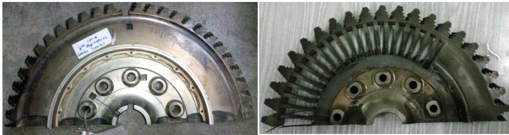
Figure 32: A portion of turbine disc exposed to 3000 hours of service life that is used for extraction of samples (a) Before and (b) After
