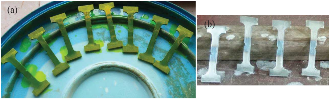
Figure 40: (a) Samples with penetrant and (b) developer applied during FLPT inspection
