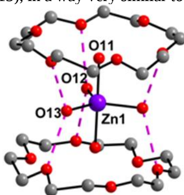
Figure 2.11. \text{Tbp}\{-\{\text{Zn}(\text{H}_2\text{O})_5\}^{2+} coordination complex cation, sandwiched between two crown ethers, in the crystal of in the crystal of compound [\text{Zn}(\text{H}_2\text{O})_5][18\text{-crown-6}]_2[\text{Mo}_6\text{O}_{19}] (3). Purple dashed lines represent the hydrogen bonds.
