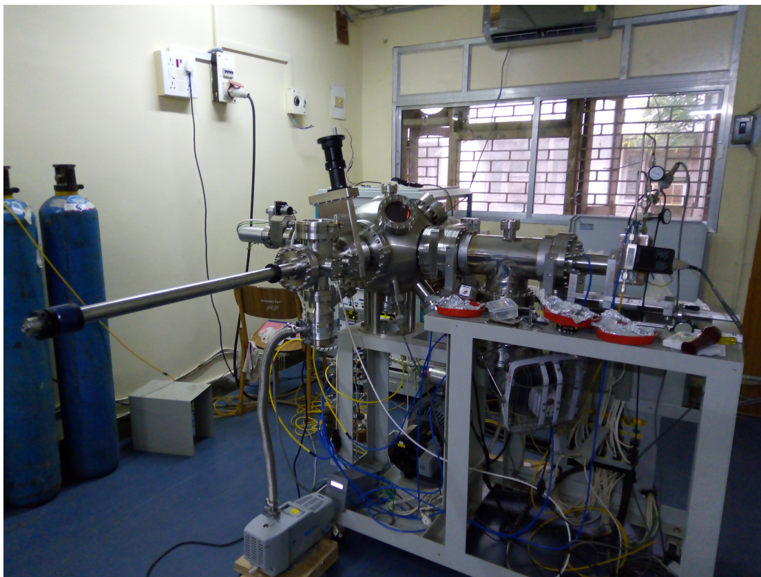
Figure 2.3: An image of nanocluster deposition system (Nanodep60).
