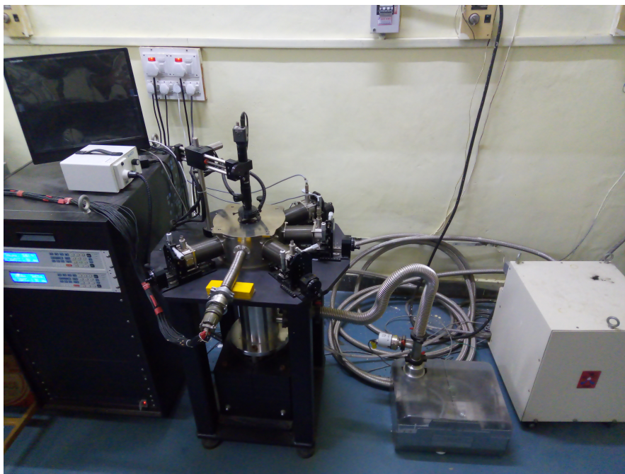
Figure 2.9: Showing the cryogenic probe station along with its accessories such as temperature controller, microscope unit, vacuum pump and closed cycle refrigerator.
