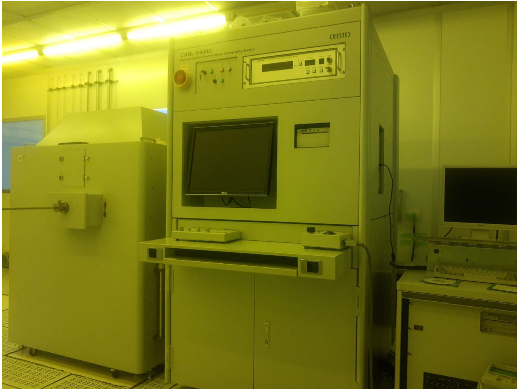
Figure 2.4: Showing the electron beam lithography system used to make MTJ photomasks.
