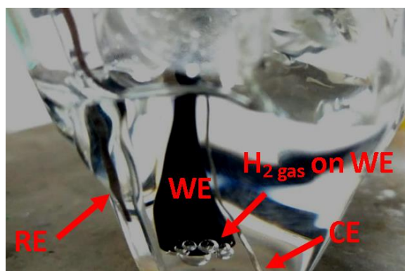
Figure 2.14. A photograph of electrochemically generated hydrogen gas on the POM-CoW(OH) 2 catalyst modified working electrode surface at neutral pH.
