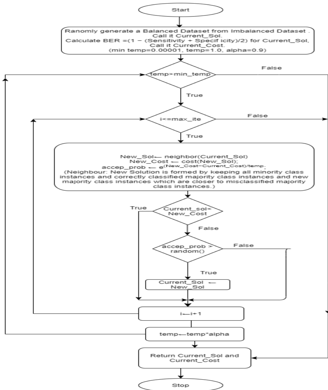
Figure 7.1: Process of Simulated Annealing based UnderSampling
