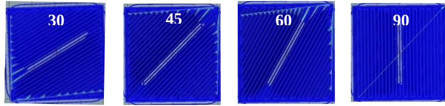
Fig. 2.25 Schematic of filling angle of rectilinear patterns
