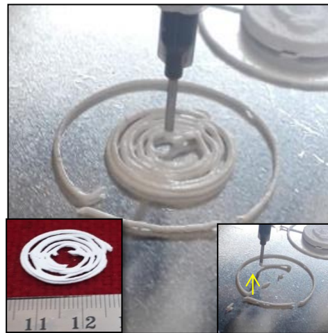
Fig. 2.20. Printing of extrudate with self-standing distance 2.0 mm
