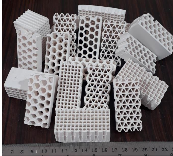
Fig. 6.2 3D printed clay honeycomb structures
