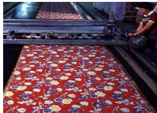
Roller printing machine and Sample of cloth printed by roller print machine
