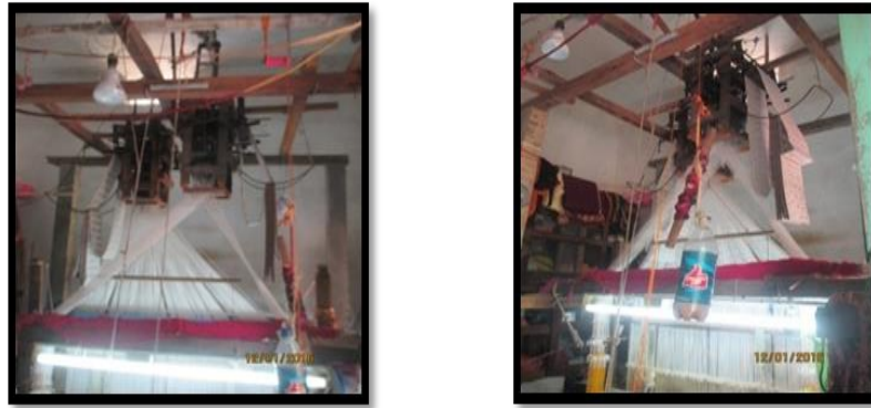
Fig.2.19: Jakard Machines with design cards Source: From field, Chirala, Prakasham District. December 2015
