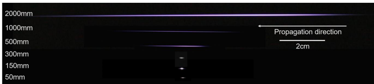
Figure 2.167: Images of the filaments imaged using the DSLR Nikon t4i camera. Exposure and gain was adjusted to capture complete spatial extent of the filaments generated using the lens with focal length=50mm, 150mm, 300mm, 500mm, 1000mm and 2000mm.
