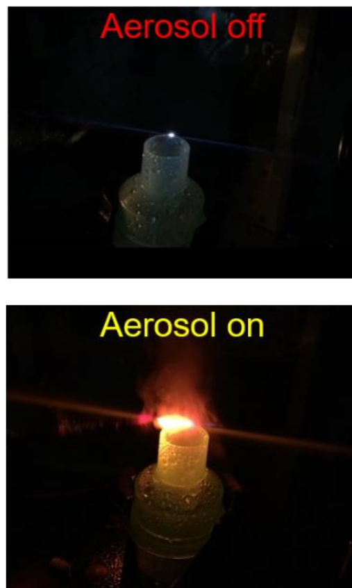
Figure 7.1: Filament aerosol interaction without (Top) and with aerosol (Bottom).
