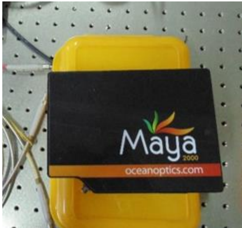
Figure 2.101: Image of the Maya 2000 spectrometer used.
