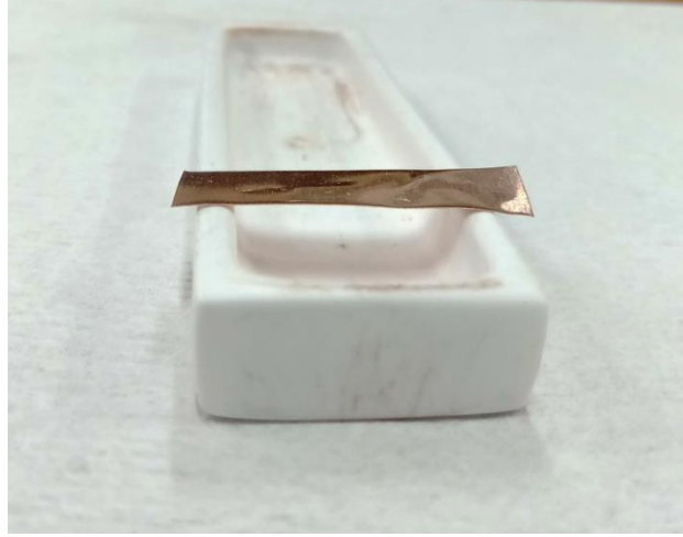
Figure 1. Copper foil placement for the non-contact annealing in argon+ hydrogen atmosphere.
