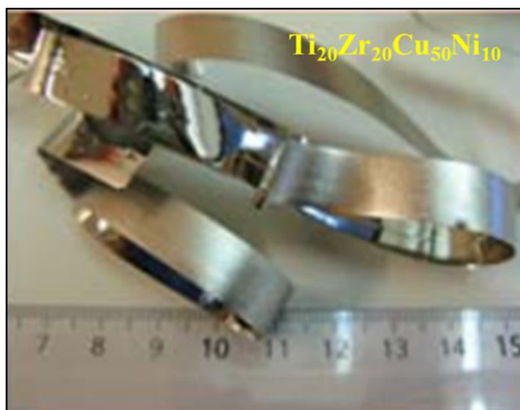
Fig.2.2 The Ti 20 Zr 20 Cu 50 Ni 10 metallic glass ribbon.
