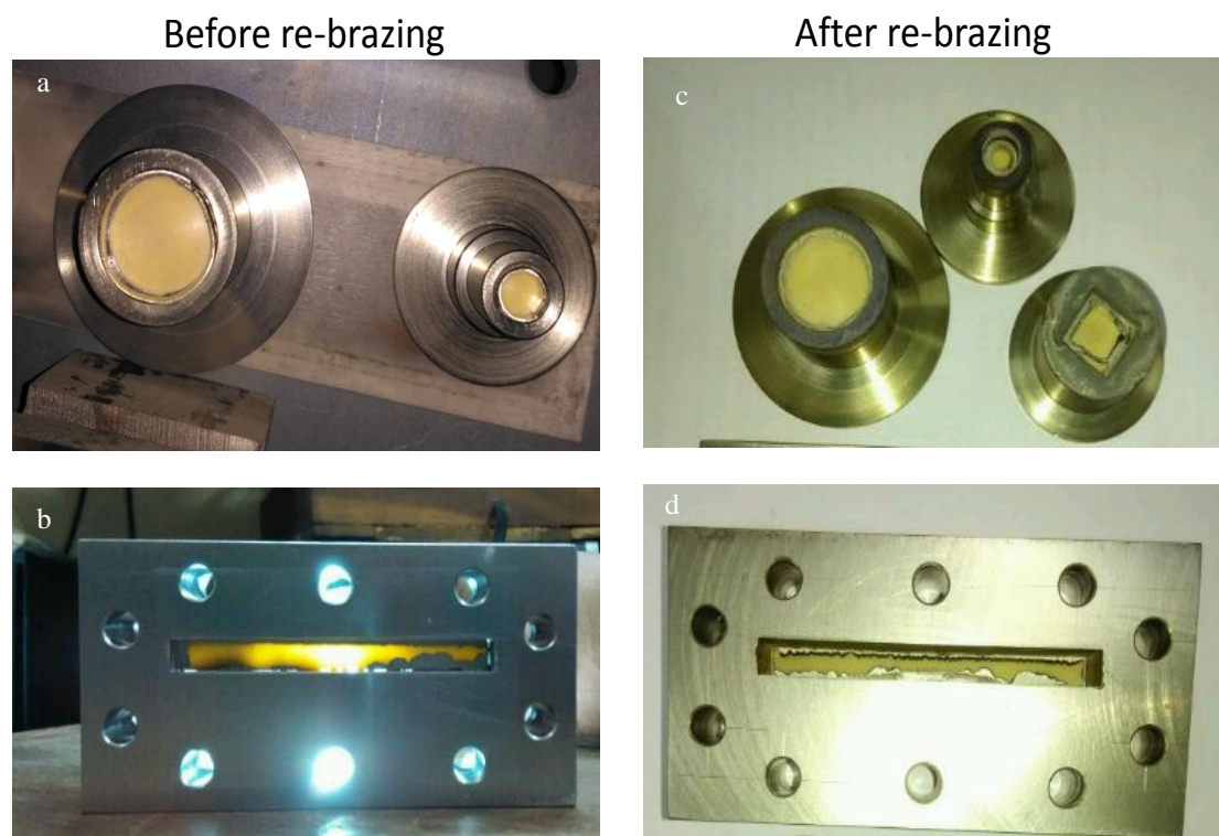
Fig 8.3 BZT samples (a,b) before re-brazing and (c,d) after re-brazing
