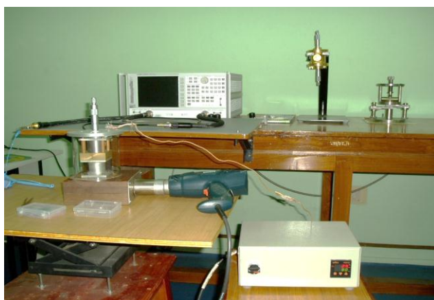
Fig 1.5 Cavity setup for measurement of temperature coefficient of resonant frequency
