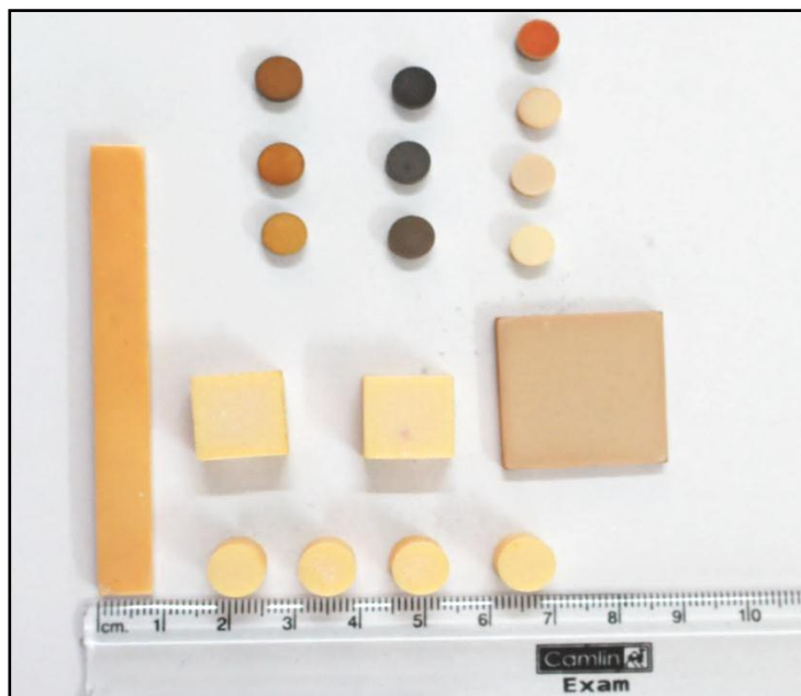
Fig 8.1 BZT samples prepared in different dimensions using various processing conditions
