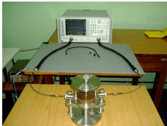
Fig 1.4. Hakki and Coleman setup to measure dielectric constant
