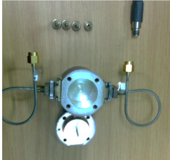
Fig 1.3 Cavity test fixture for TE_{01\delta} mode dielectric resonator method
