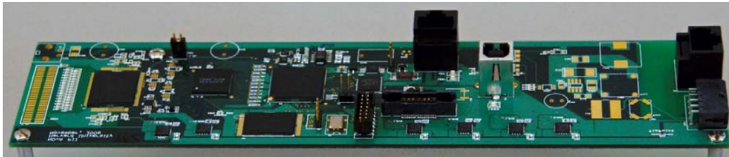
FIGURE 2.14: Layout of the FEB. Major components are the carrier board connector location at the left, which brings the APD signals to the NOvA ASIC, which performs integration, shaping, and multiplexing. The chip immediately to the right is the ADC to digitize the signals, and FPGA for control, signal processing, and communication.
