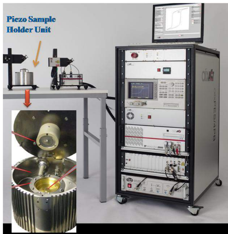
Fig. 2.17 Polarization and strain versus electric field measurement with aixACCT system with Piezo sample holder unit (PSHU) [28].
