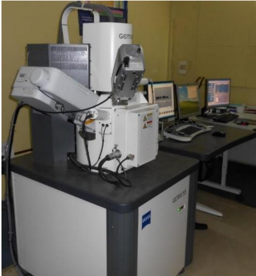
Fig-2.11: A picture of FESEM system at SoP, UoH [18].
