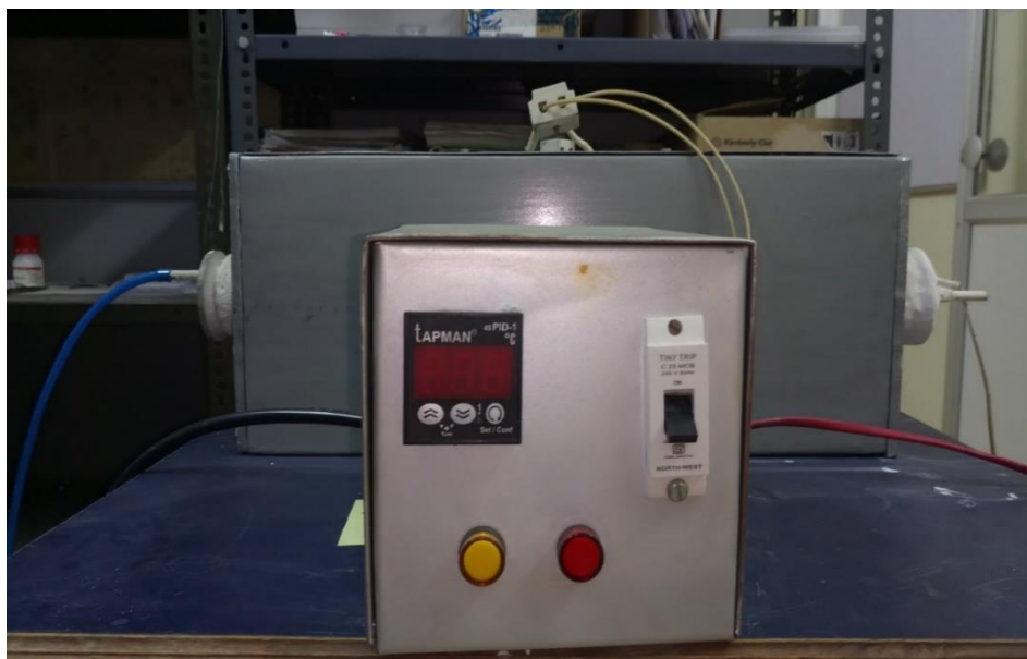
Fig-3.11: Furnace used for annealing of the films.
