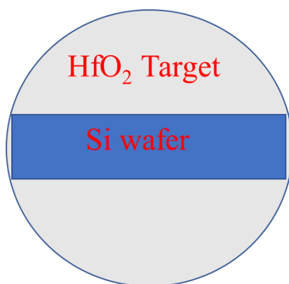
Fig-6.1: Schematic diagram showing of 30 % of Si coverage on the HfO 2 target.
