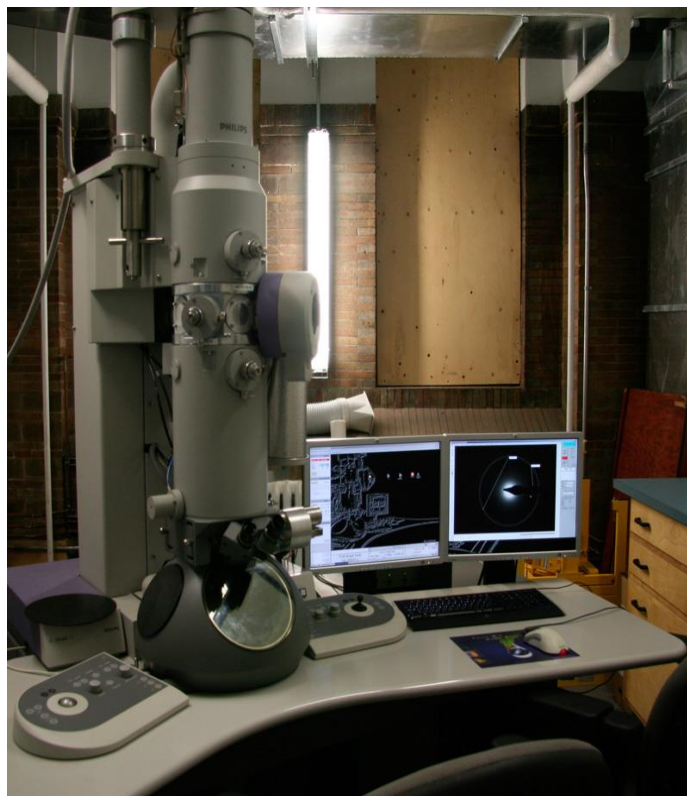
Fig-2.13: TEM (FEI Technai G2S- Twin 200 keV) instrument at CNF, UoH [21].
