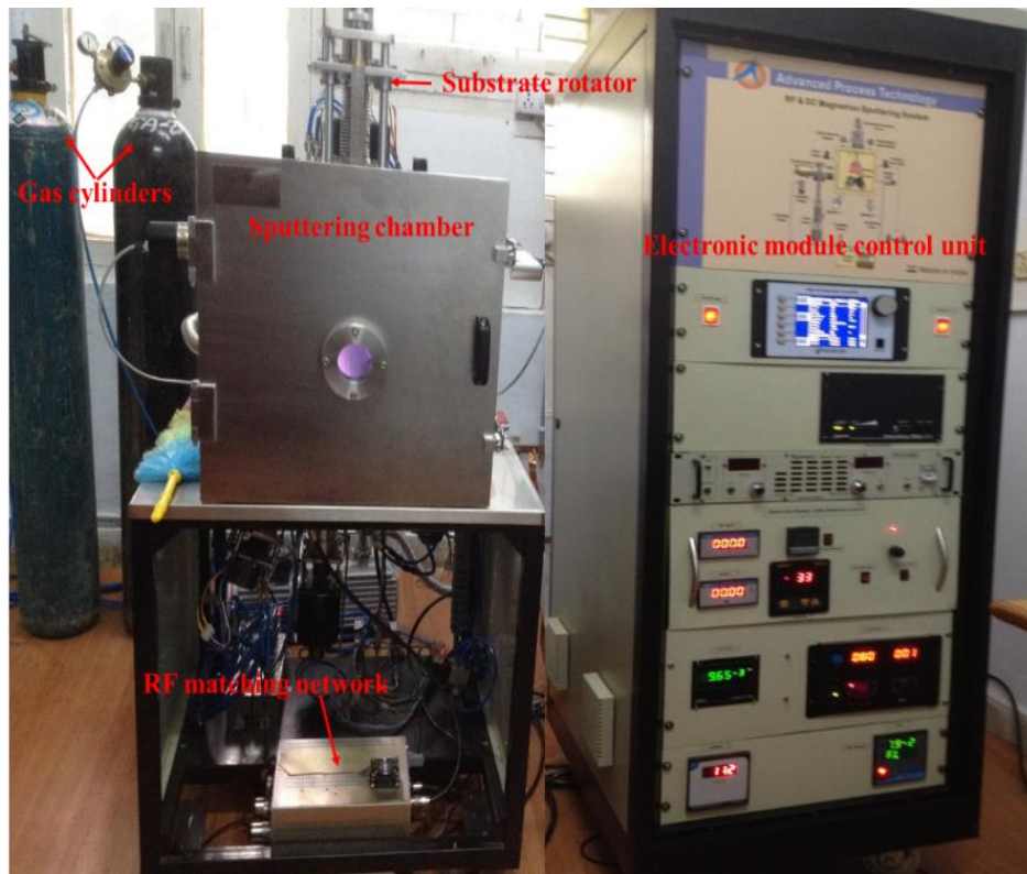
Fig-2.2: RF and DC magnetron sputtering system installed at SOP, UOH.
