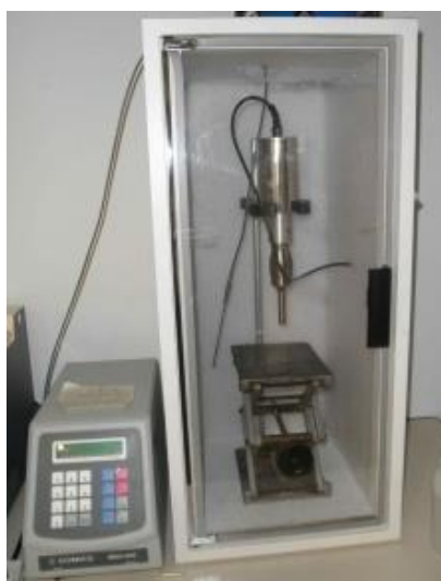
Figure 3.3. Photograph of the probe sonicator used in this thesis work.
