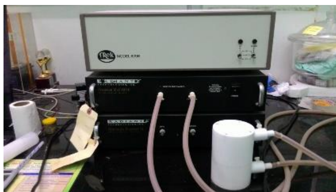
Figure 3.5. Photograph of the P-E hysteresis measuring instrument used in this work.
