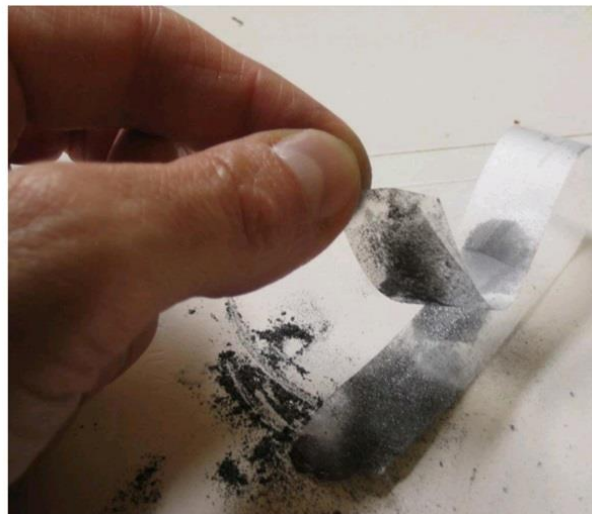
Fig.1.2. Mechanical cleavage process by using the scotch tape [50].
