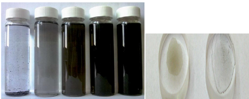
Fig. 1.4 (a) From left side to right side: pristine graphite and exfoliated graphene as achieved by tip sonication for 5, 15, 30 and 60 minutes, in o-DCB (b) Picture of the \frac{1}{2} -inch fused silica windows with GO and rGO coatings [26, 31].
