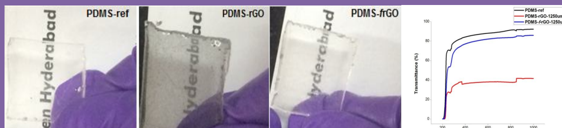
Fig. 6.2.7 Photography images of (a) PDMS-ref (b) PDMS-rGO and (c) PDMS-1,4-D-rGO and (d) UV-visible spectra of PDMS-ref, PDMS-rGO and PDMS-1,4-D-rGOnanocomposites.
