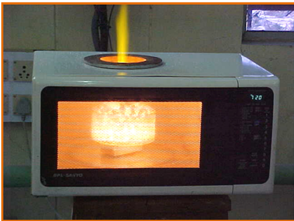
Figure 1.8: Combustion reaction performed in microwave oven during the preparation of catalysts.
