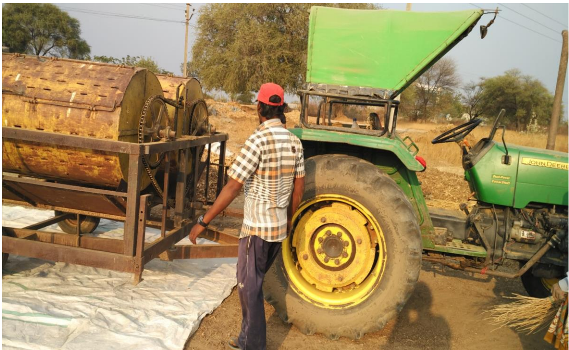
Plate-8 Operator using machinery for polishing turmeric
