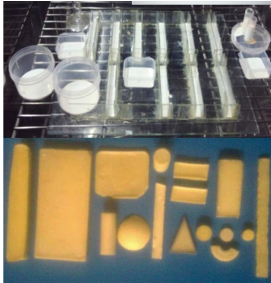
Fig. 5.7 Zr_{0.8}Sn_{0.2}TiO_4 gel after casting in plastic and glass moulds
