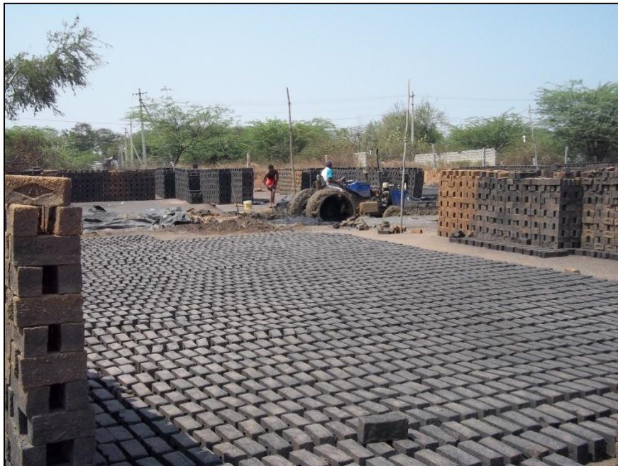
Picture 4.4: Bricks arranged in herring bone pattern
