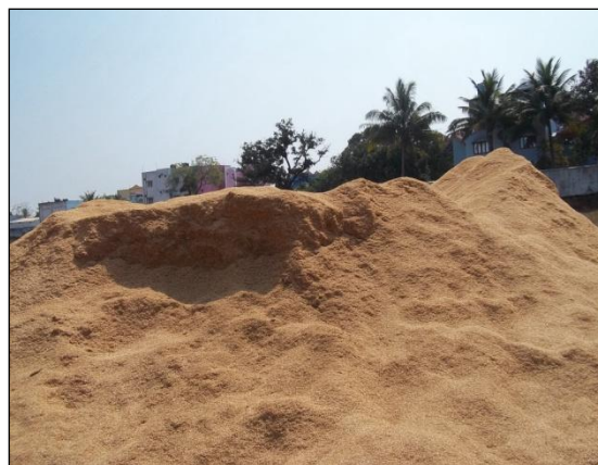
Picture 4.6: Paddy husk used for making fly ash bricks
