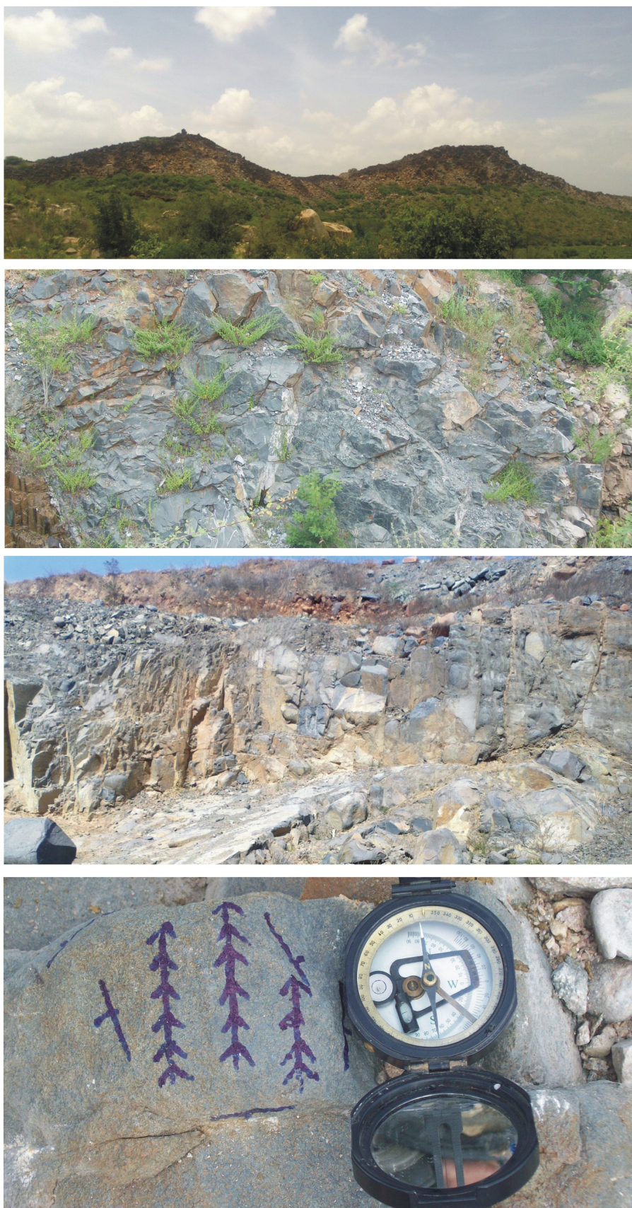
Figure 2.4. Field photographs of well exposed and insitu outcrops and hand sample collection for paleomagnetic studies using Brunton compass.
