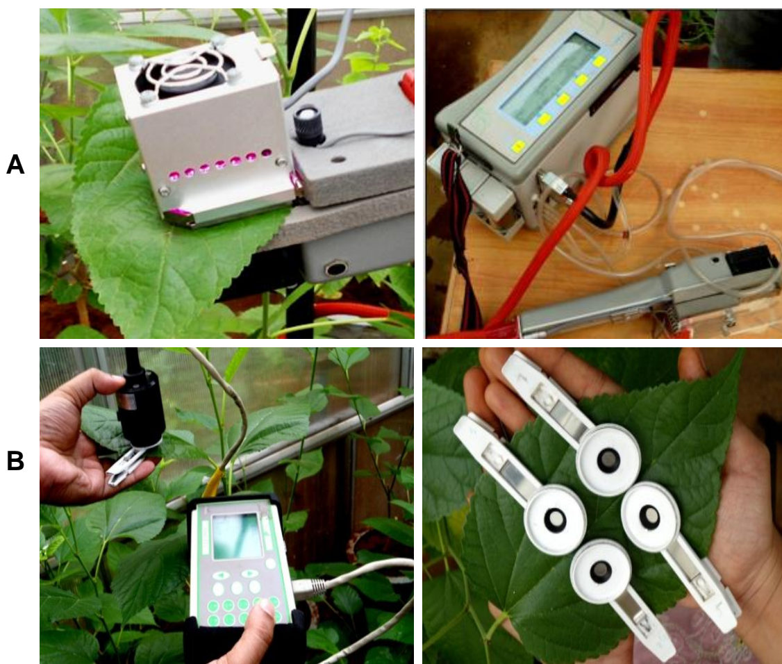
Fig 2.2 Infra red gas analyzer (IRGA) used for the measurements of photosynthetic leaf gas exchange physiology (A) and Handy PEA used for measuring PS-II efficiency (B) in mulberry.
