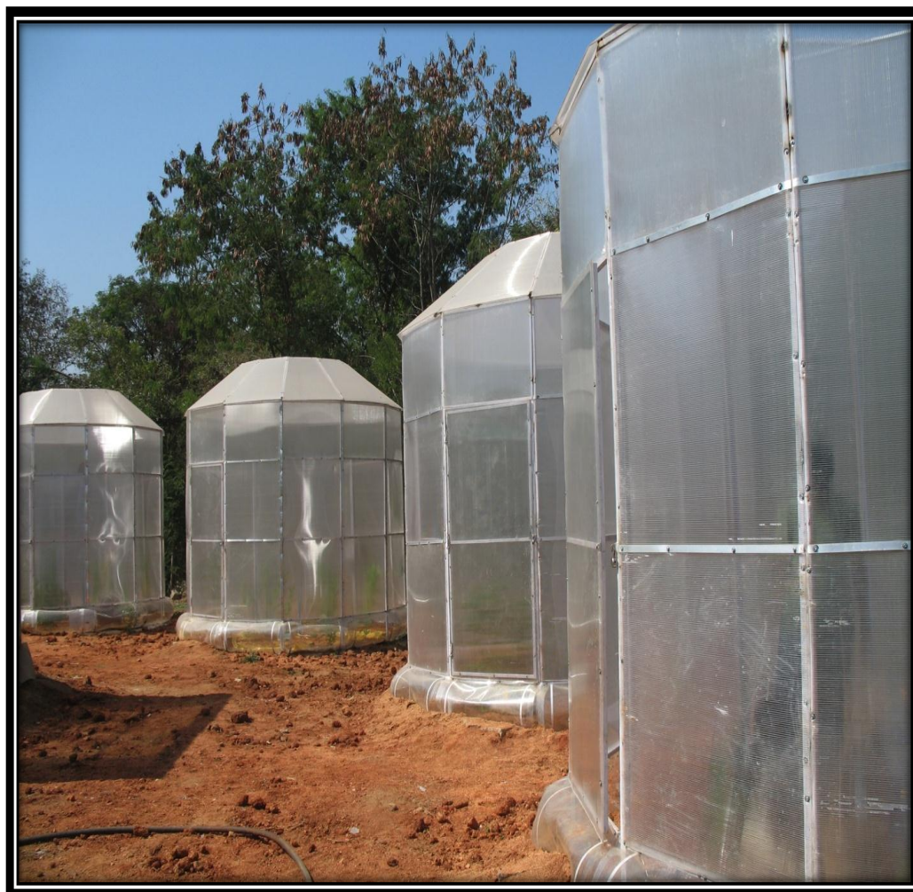
Fig 2.1 Experimental facility: OTCs established in the botanical garden of University of Hyderabad for [CO 2 ] enrichment studies.
