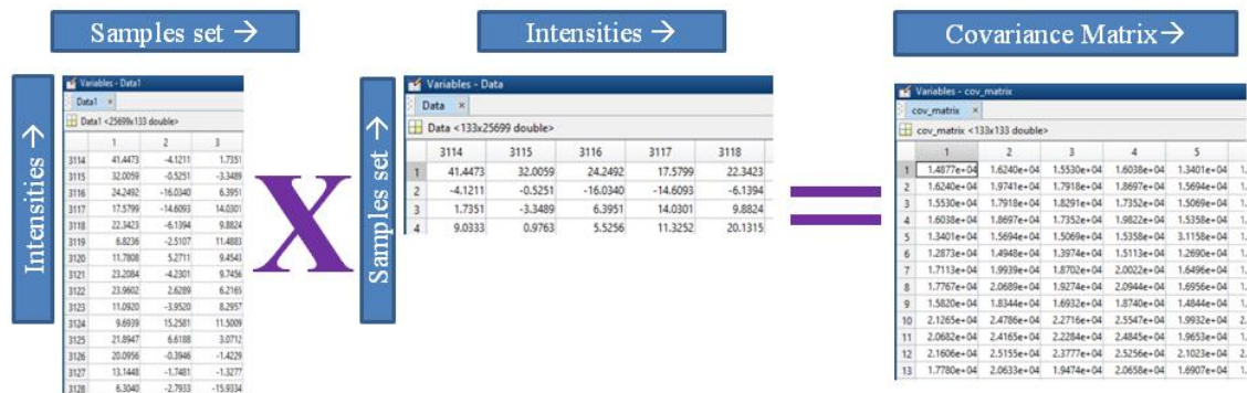
Figure 9. Calculation of covariance matrix using mean centered data matrix.
